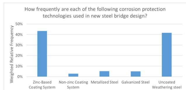
**Figure 2. Relative popularity of steel bridge corrosion protection technologies.<sup>1</sup>**
