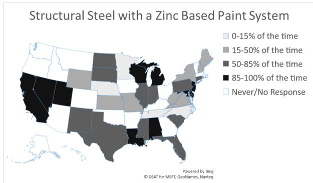
**Figure 3. Use of 3-coat, zinc-based coating system for steel bridge corrosion protection.<sup>1</sup>**
