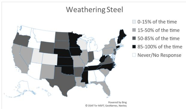
**Figure 5. Use of uncoated weathering steel bridge designs.<sup>1</sup>**
