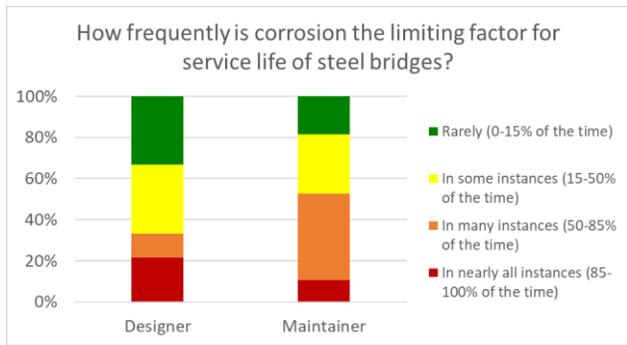
**Figure 1. Survey results regarding corrosion as a life limiting factor for steel bridges.<sup>1</sup>**
