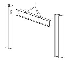
The beam is lifted in place by a crane. Ironworkers will align the beam and install the connection bolts.
