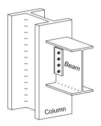
The final installed connection.
