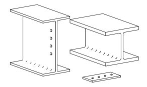
Material cut to length. Holes are drilled or punched.
