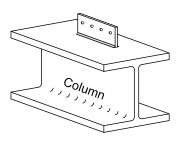
The plate is welded to the column.
