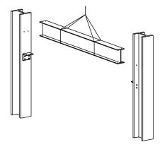
The beam is lifted in place by a crane. Ironworkers will align the beam and install the top angle and connection bolts.
