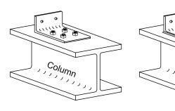
The angle is bolted or welded to the column.
