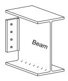
The plate is welded to the beam.
