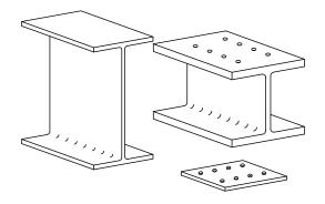
Material cut to length. Holes are drilled or punched.
