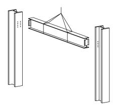
The beam is lifted in place by a crane. Ironworkers will align the beam and install the connection bolts.
