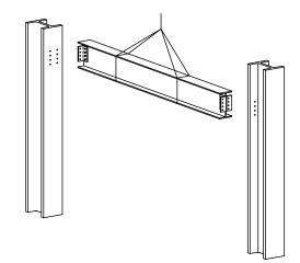
The beam is lifted in place by a crane. Ironworkers will align the beam and install the connection bolts.
