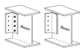
Angles are either bolted or welded to the beam.
