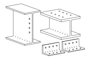
Material cut to length. Holes are drilled or punched.
