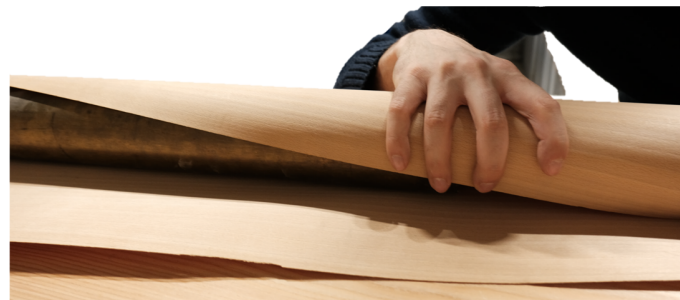
Figure 4: Rolling-up of the 0.6 mm beech veneer sheets around the circular hollow profile.
