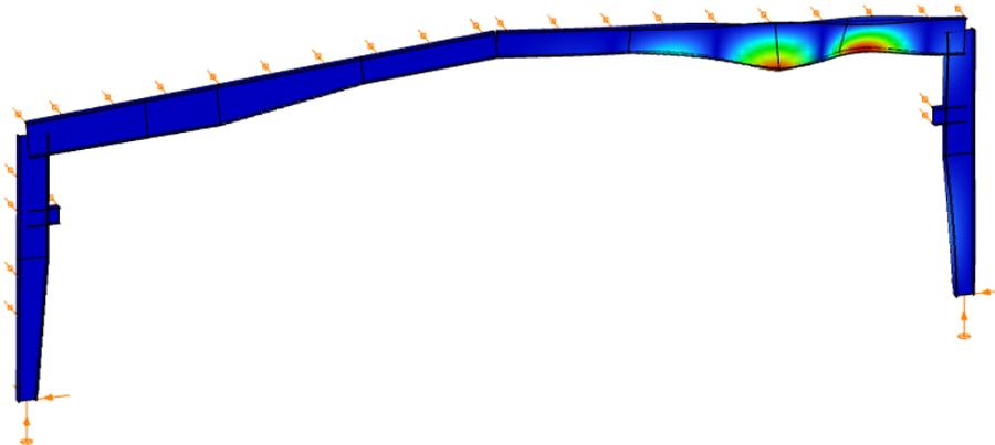
Figure 6: Out-of-plane buckling mode for the right-hand column in the clear-span crane-building frame
