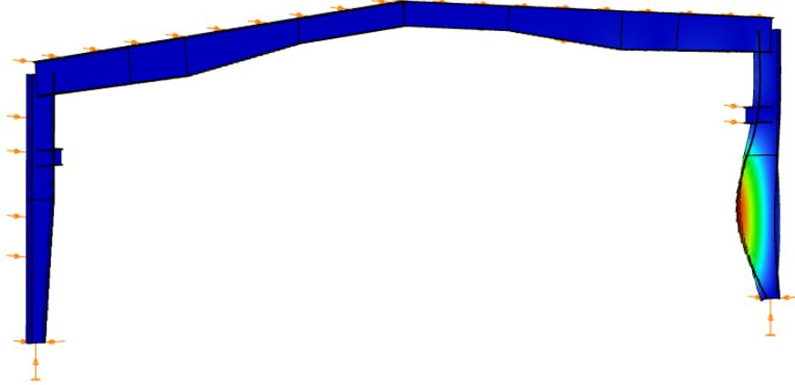
Figure 5: Out-of-plane buckling mode for the right-hand column in the clear-span crane-building frame
