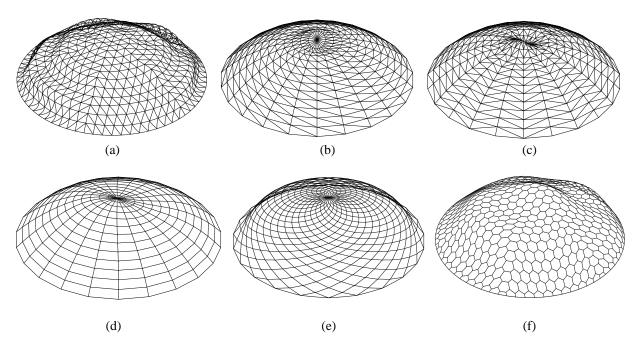
Figure 9: First buckling mode for the dome configurations: (a) Kiewitt dome (b) Schwedler monoclinal dome (c) Schwedler bidirectional dome (d) Radial rib dome (e) Lamella dome (f) Hexagon dome
