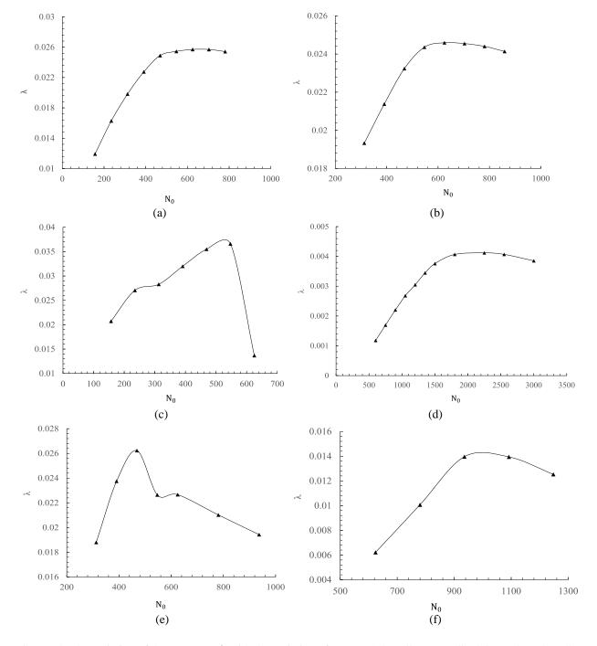
Figure 14: The variation of the parameter  $\lambda$  with the variation of N<sub>0</sub> : (a) Schwedler monoclinal dome (b) Schwedler bidirectional (c) Radial rib dome (d) lamella dome (e) Sunflower dome (f) Hexagon dome
