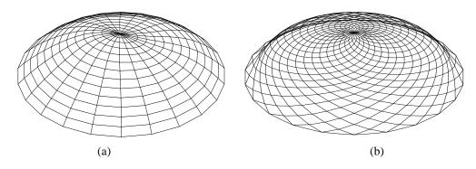
Figure 4: First buckling mode is different for the configurations even though the edge valencies are the same, indicating the influence of member orientation on global stability: (a) Radial rib dome (b) Lamella dome
