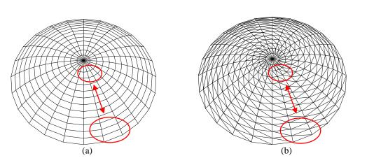
Figure 6: Variation of member length from apex to support for dome configurations with radial members: (a) Radial rib dome (b) Shwedler monoclinal dome
