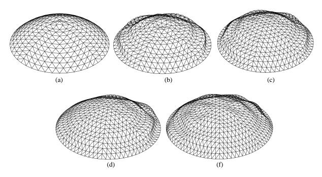
Figure 12: The first buckling mode shape for the Kiewitt dome with different face valency of the cell by varying the value of M: (a) M = 4 (b) M = 5 (c) M = 6 (d) M = 7 (e) M = 8
