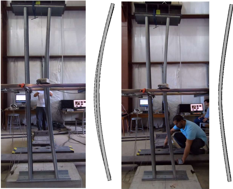
Figure 15: Comparison of failure modes: (a) 97 mil E0.0 (b) 54 mil FB
