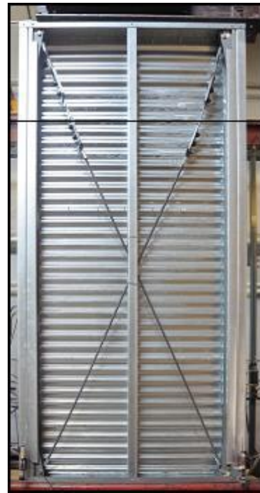
Figure 8: Layout of the shear walls structure (a) The back-view of CFS shear wall using EDB (b) The photograph of CFS shear wall using EDB
