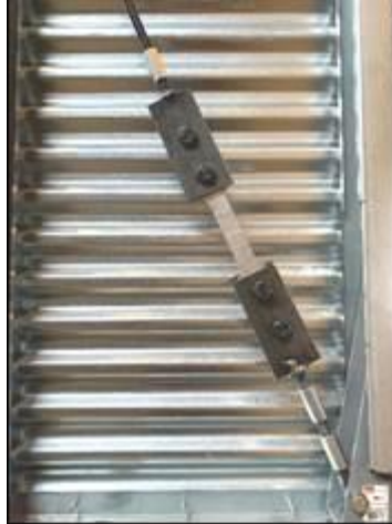
Figure 2: The photograph of energy dissipation bracing
