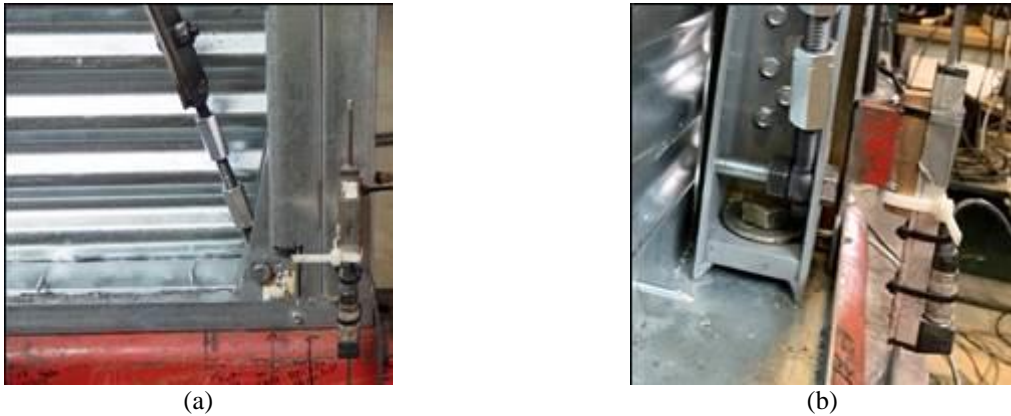
Figure 5: The connection between hold-down and EDB (a) front view; (b) side view
