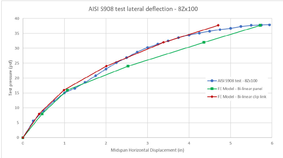
Figure 6: Comparison of lateral deflection for 8Z100 - AISI S908 test versus FE Model
