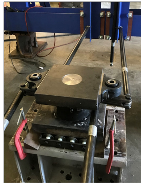
Figure 5: Bearing boundary condition detail, concept (left) and implementation (right). The spherical bearing is excluded in the photo to show the counter-bore. Additionally the roller pack is chocked in the photo to prevent incidental movement while installing the test specimen.
