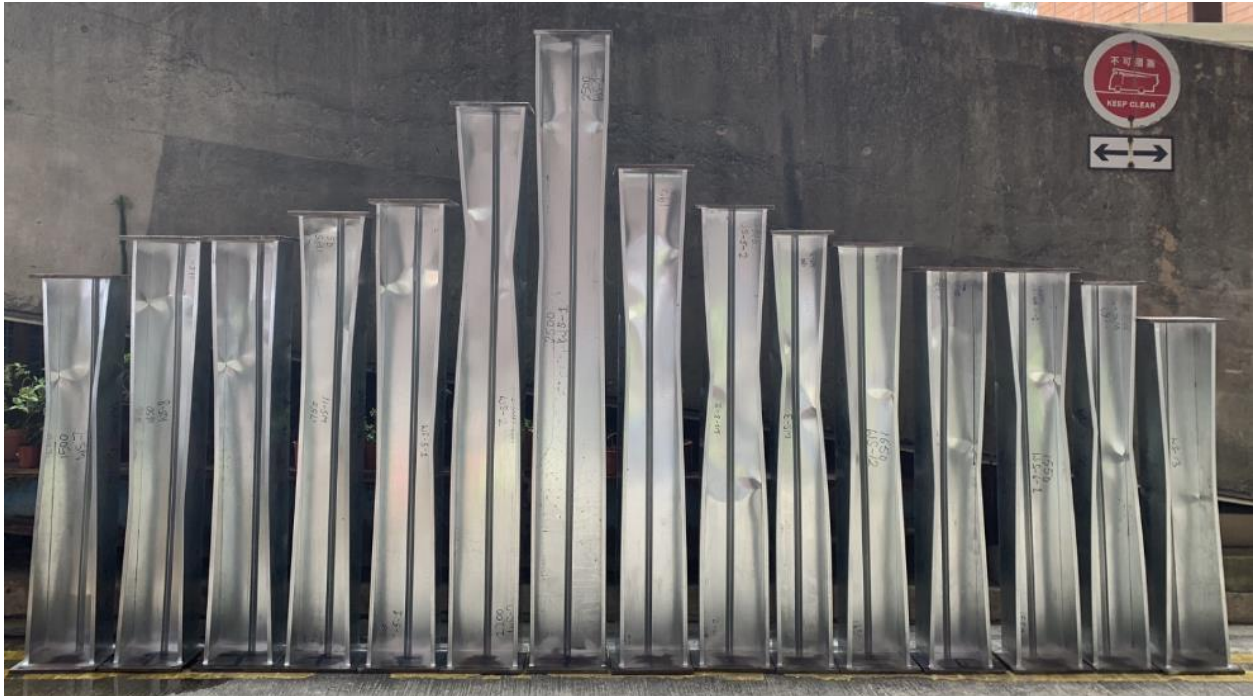
Figure 19: Deformed configurations of all WSLC specimens after the full removal of the applied load.
