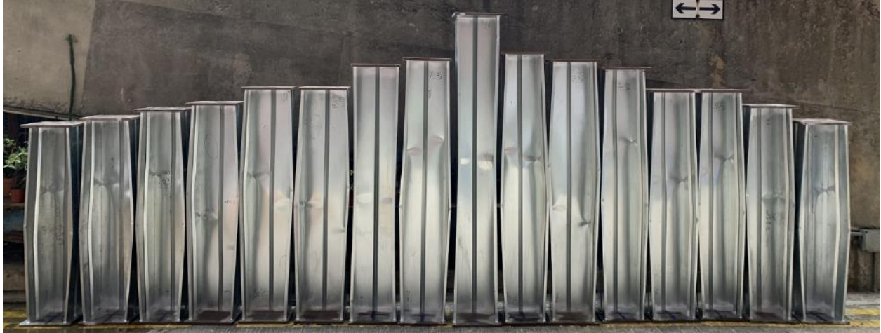
Figure 18: Deformed configurations of all WFSLC specimens after the full removal of the applied load.
