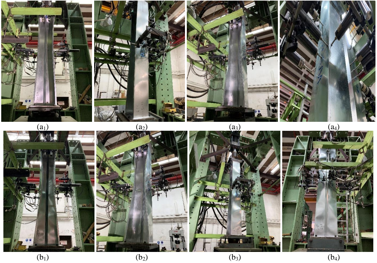
Figure 16: WSLC-13 column deformed configurations (a) prior to collapse (ascending branch) and (b) at the onset of collapse (failure mode).
