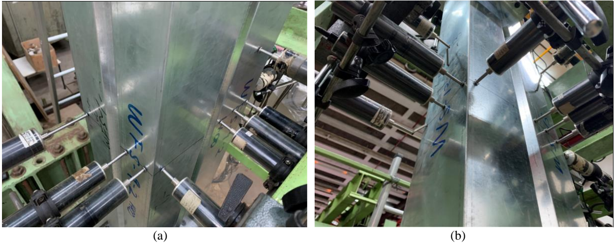
Figure 5: Transducer arrangement at the mid-height cross-section of the (a) WFSLC and (b) WSLC specimens.
