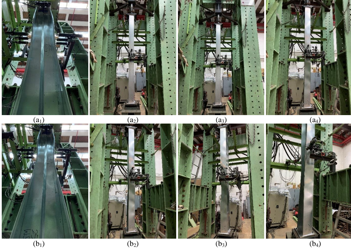
Figure 13: WSLC-1 column deformed configurations (a) prior to collapse (equilibrium path ascending branch) and (b) at the onset of collapse (failure mode).
