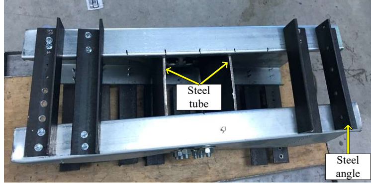
Figure 4: Connection details of the two joists (photo taken after test)
