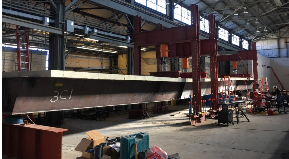
Figure 12 – Continuous Girder Configuration Test Setup – Tub 3
