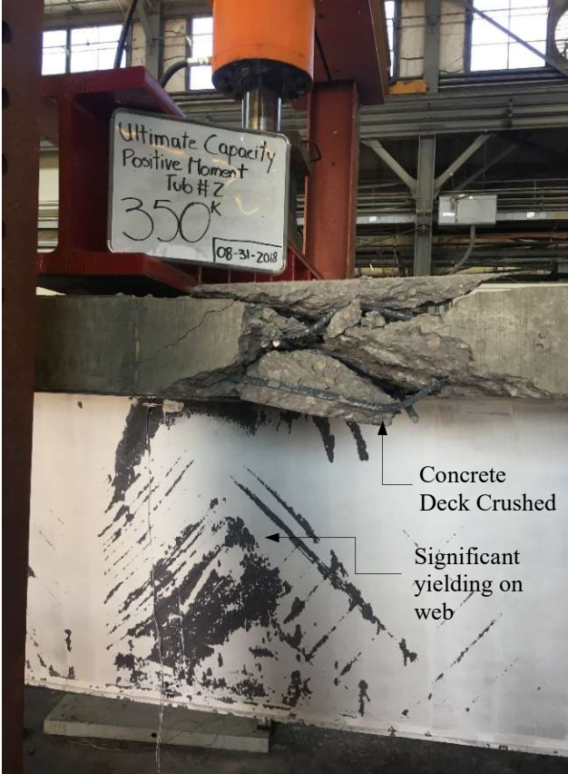
Figure 15 – Failed Section under Positive Moment Demands – Tub 2
