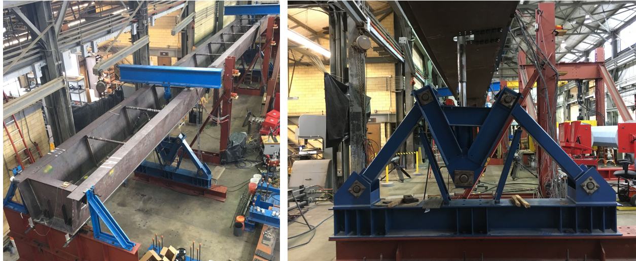
Figure 4 – a) Test Setup with Unbraced Tub 1, b) Gravity Load Simulator (GLS)
