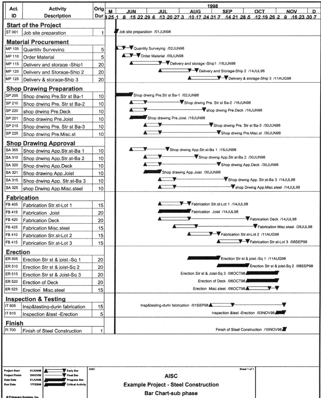
Figure 2.6 Bar chart on the basis of sub-phases
