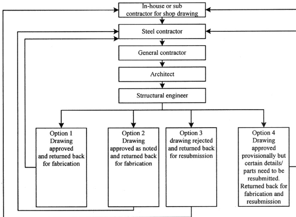
*Figure 2.8 Shop drawing approval process*
