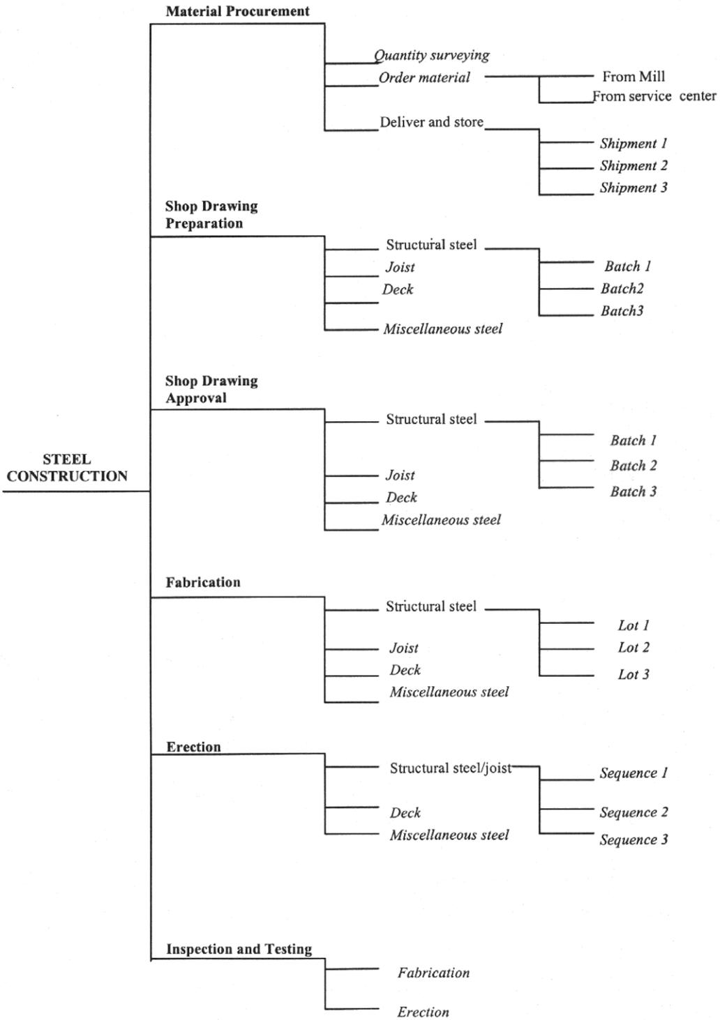
Figure 2.1 Work breakdown structure (WBS)
