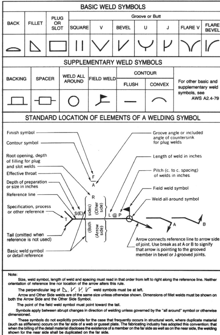
Figure 2.14 Welded joint symbols
