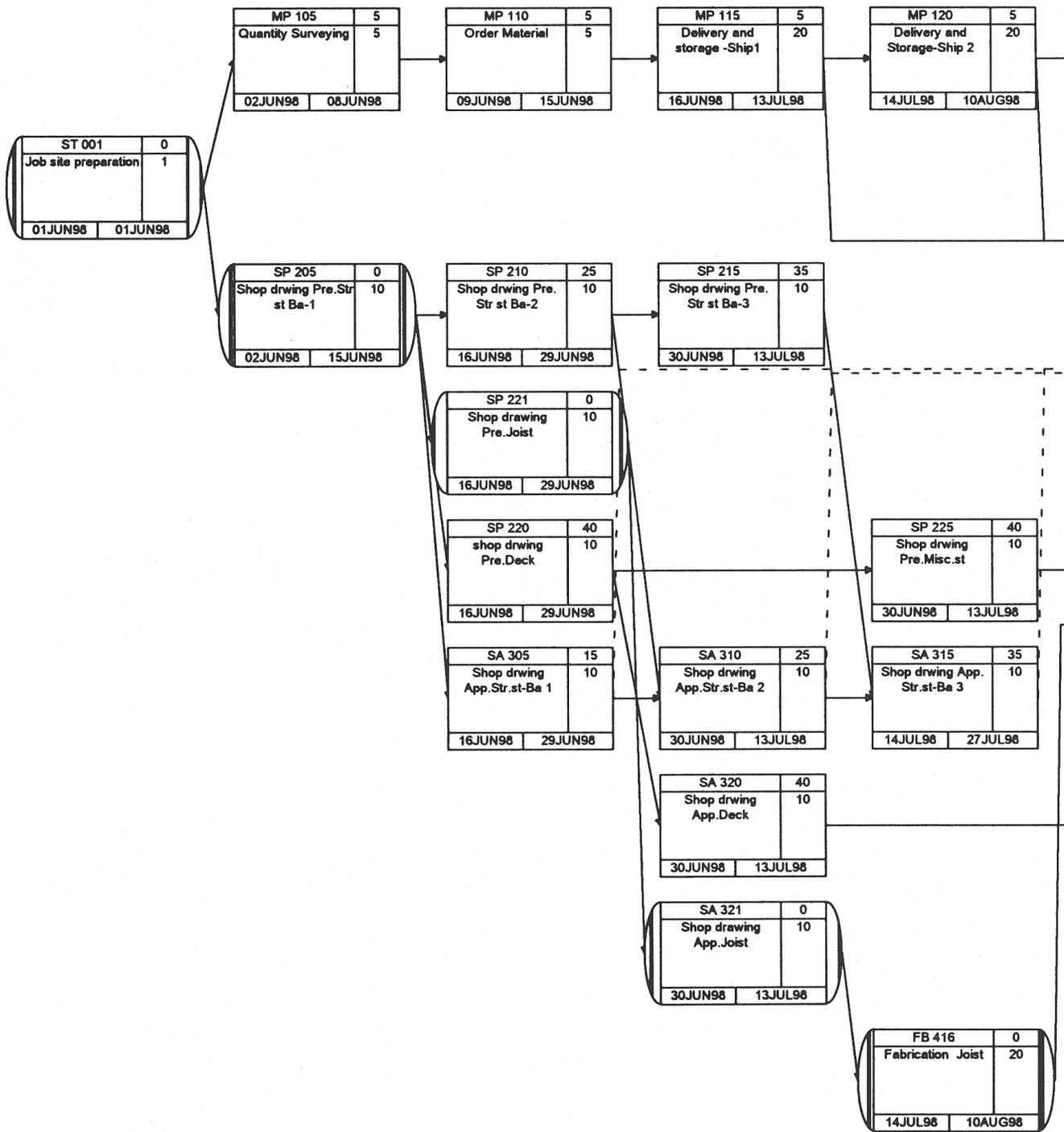
Figure 2.2 Detailed CPM diagram
