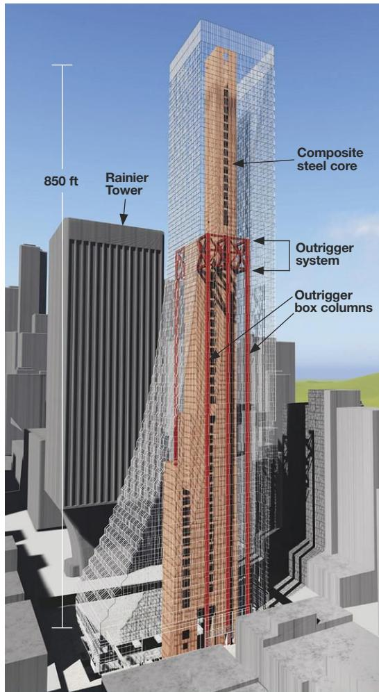
**TALL AND SLENDER** Rainier Square Tower needs a system of outrigger trusses to reduce its sway.
