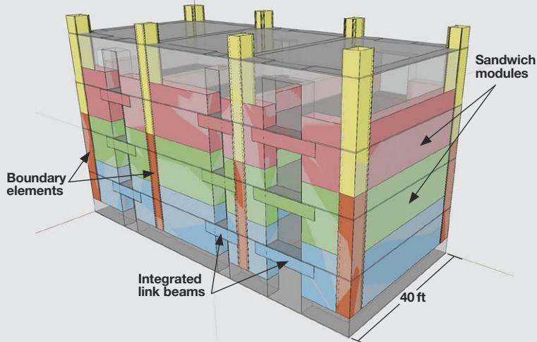
**STACKING UP** The plan is to stack and field-weld the steel modules. When the erector finishes four levels, crews will add concrete.
